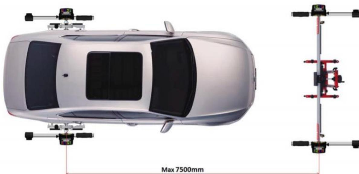
The first integration available is with AUTEL brand and allows to quickly and precisely align the panel placed in front of the vehicle with the car thrust angle.
